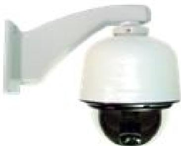
TELECAMERA SPEED DOME 30X, 470 LINEE DAY & NIGHT (FILTRO MECCANICO RIMOVIBILE) MOTORIZZATA 1/4" X ESTERNO COMPLETA DI CUSTODIA IP-66 IN ALLUMINIO VENTILATA E RISCALDATA ANTIAPPANNAMENTO,CUPOLA IN ABS ANTIVANDALO
